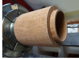
Sand the edge with fine sandpaper, \sim 320 grit.
