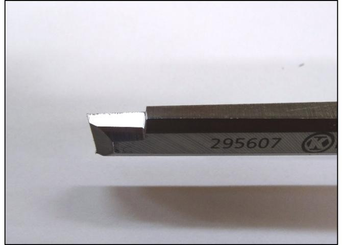
Figure 7. Bottom/Left Side View of Chisel Regrind
