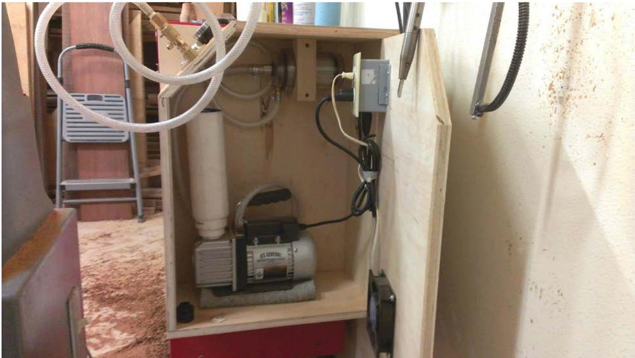
Figure 1. Filter in place on pump.
