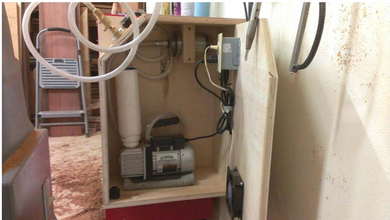
Figure 1. Filter in place on pump.
